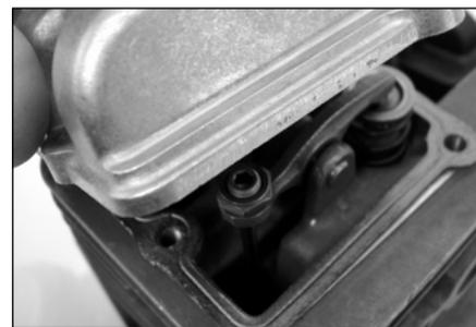
2. Loosen adjuster locknut so that the 2.5 mm Allen socket head adjustment screw can turn freely.
