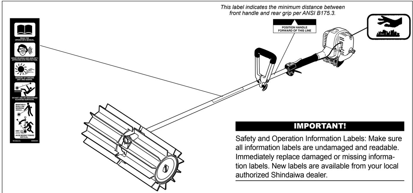
This label indicates the minimum distance between front handle and rear grip per ANSI B175.3.
